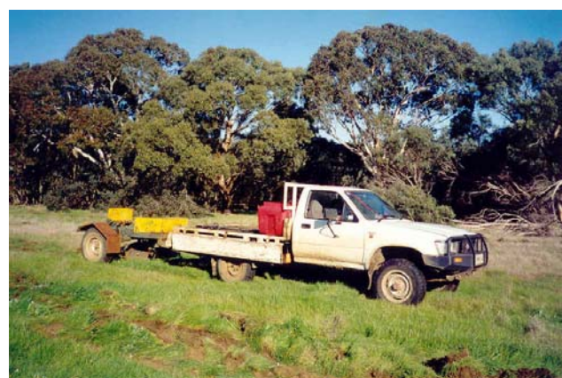
Malcolm’s ute and trailer mounted tree direct seeder.
